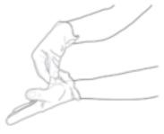
Pinch one glove at the wrist level to remove it, without touching the skin of the forearm, and peel away from the hand, thus allowing the glove to turn inside out
